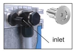
In case, install a small flange connection KF DN 16 (thread G1/8") instead, see "Accessories", pg. 46).
