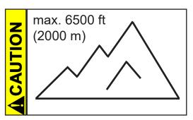
If the pump is installed at an altitude of more than 6500 ft (2000 m) above mean sea level, check compatibility with applicable safety requirements, and adopt suitable measures. There is a risk of the motor overheating due to insufficient cooling.
