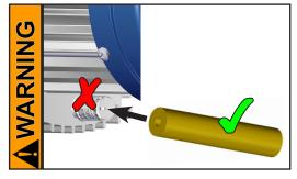
Connect a gas-tight exhaust line at the pump outlet (see above) if necessary. Always vent exhaust gases appropriately (e.g., into a fume hood). ways be free of obstructions (no back pressure) to ensure an unimpeded discharge of gas. The cross-section of the outlet tubing must be at least the size of the pump's exhaust connection.
