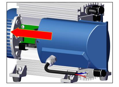
Assemble cover after replacing the fuse.
