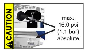
Check compatibility with the maximally permitted pressure at outlet and the maximum pressure difference between inlet and outlet ports.
