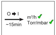
A warm up period (approximately 15 min.) is required to ensure that the rated ultimate vacuum and pumping speed are attained.
