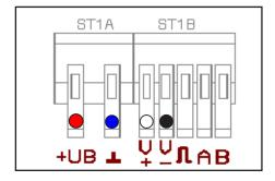
→ Connect the black and the white wire accordingly to the terminal board ST1B (see table above).
