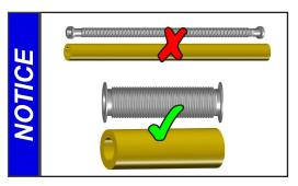
Use connecting hoses with large diameter and keep them as short as possible to avoid flow losses. Locate the pump as closely as possible to the application.
