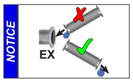
Always install outlet tubing descending from the pump to avoid backflow of condensate towards the pump.
